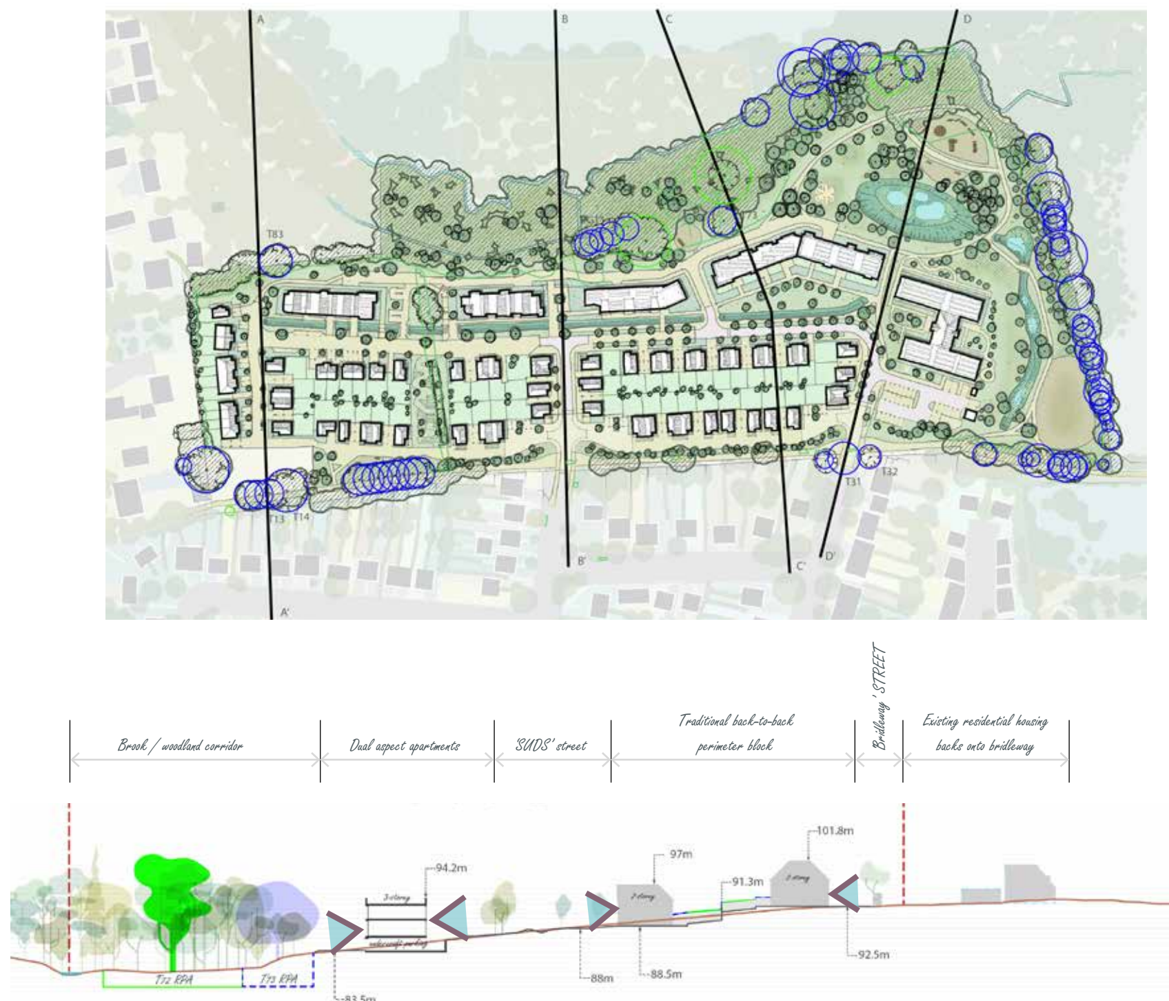
Figure 28: Section CC' showing block relationships
